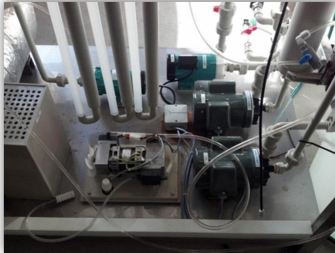
Figure 6 - 4 green Iwaki pumps and KNF vacuum pump (with cover removed)
