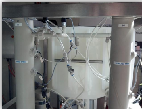
Figure 5 - PVC process piping and polyurethane vacuum tubing
