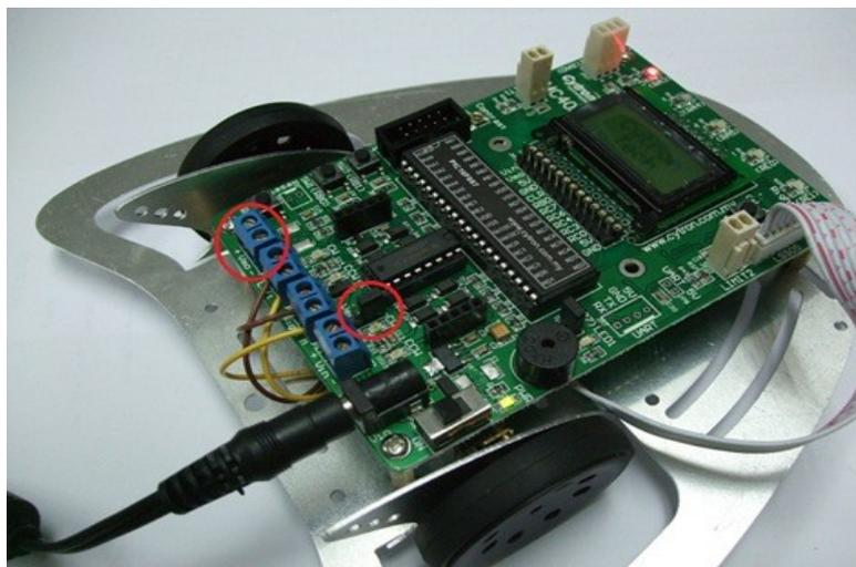
Motor Power Input Terminal and Selection Jumper
