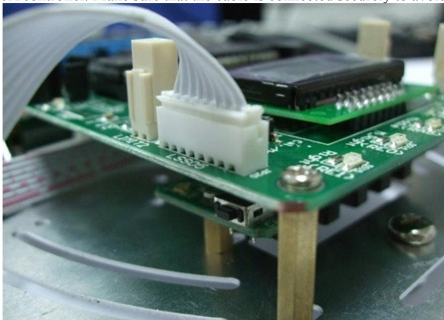
LSS05 cable connected to MC40A Controller Board
