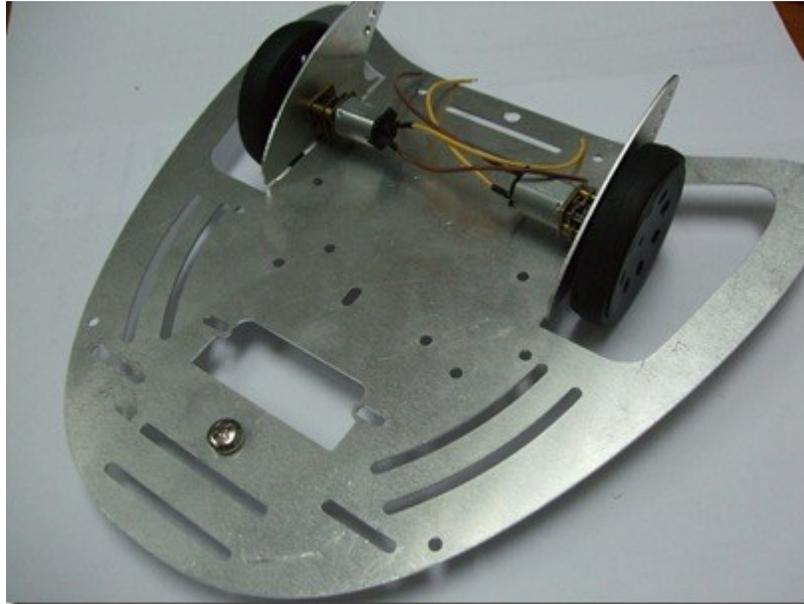
Base completed with SPG10 motors, Wheel and Screw Castor
