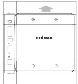
2. Attach the two magnetic wall mount strips to your wall using the included screws, as shown below.
