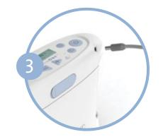
Connect the AC Power Supply cord to the Inogen One G<sub>3</sub>.
