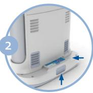
Insert the Inogen One® G<sub>3</sub> battery by sliding battery into place until the latch returns to the upper position.
