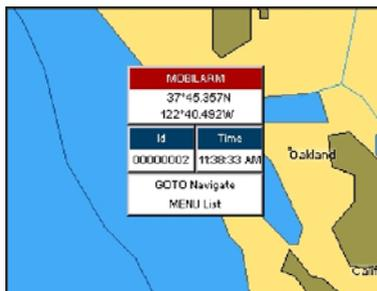
Figure 16.3.0a - Example of PTX warning window
