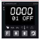
The F-key opens the profiler control menu in the lower display line. The display will show "P:" followed by the actual state. Depending on the configuration, the menu allows the user to select RUN/ stop or RUN/stop/reset with the UP/DOWN-keys. Press ENTER to make the selected state active.
