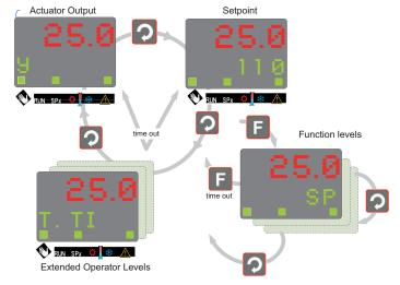
The content of the extended operating level and the function level is based on configurations made with the configuration utility ChromaloxPro. Parameters used frequently or important measured values can be placed into the extended operating level.
