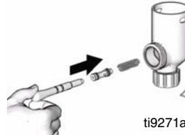
2. Insert spring guide with o-ring into flow adjustment nut. Make sure the protruded end of the guide points out as shown.
