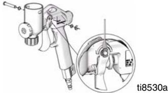
6. Unscrew nozzle and remove it from gun.
