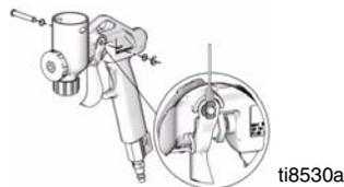
9. Pull trigger and replace nozzle.
