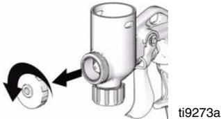
7. Hold needle securely in place so it does not turn while turning flow control clockwise until needle is disengaged from thread and released. Pull needle and o-rings out front of gun.
