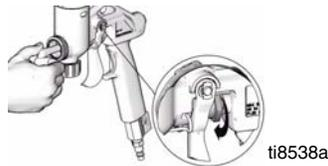
6. While pushing needle into gun, turn flow adjustment nut counter-clockwise to tighten needle.
