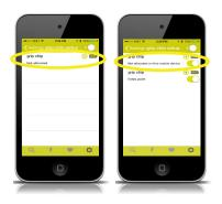
Note: You will see "Not allocated on this device" if you attempt to connect to a grip chip that has been previously programed with a favorite using a different Apple device than the one you are currently using. In this case, you can still re-configure the chip, but will not see how it was previously configured.
