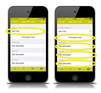
Tapping "Find grip chip" will cause the selected grip chip to illuminate and make a sound. This allows easy confirmation of which grip chip is connected.
