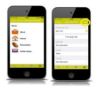
After selecting a favorite to assign, tap "Save" when arriving back to the "grip chip info" screen. The grip chip is now shown with its name, assignment, number and battery level.
