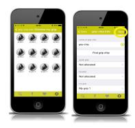
After selecting a **my grip** to assign, tap "Save" when arriving back to the "grip chip info" screen. The grip chip is now shown with its name, assignment, number and battery level.
