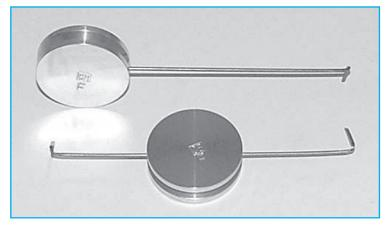
In the photo (left), it can be seen that the Thumbturn is sitting half way along the length of the Picking Wire, changing from a left handed pick to a right handed pick.
