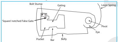
**3. ii**] A Procedure of Picking a Lever Lock with V Notched False Gates.
