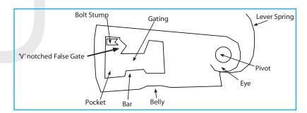
**3. iii**] A Procedure of Picking a Lock with Square False Gates.
