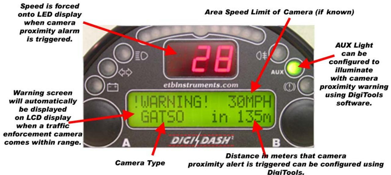
The following instructions assume that you have connected you DD2-Lite to a laptop PC and have already configured the DD2-Lite to suit your vehicle (speed, rpm, gear ratios, general warning alarm settings etc.).
