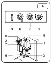
whereas the solenoid valve will bleed the air off the final manifold and head, thus favoring next compressor start.
