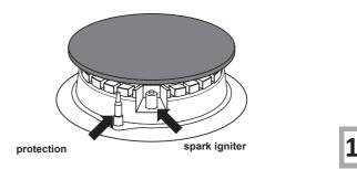
Hold the burner's control knob depressed for approx. 10 seconds in Burner ON large flame position. This way, you activate the protection device.
