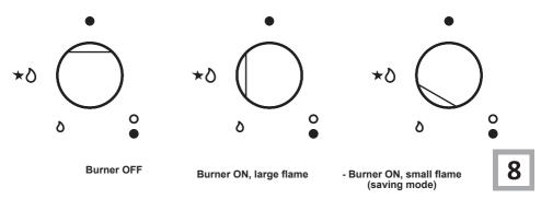
See also fig. 8 for various operating options (flame size selection); the burner should be set at a large flame during the initial phase of cooking to bring the food to boiling, and then the knob should be turned to the saving flame position to maintain the cooking. It is also possible to adjust the flame size stepless.
