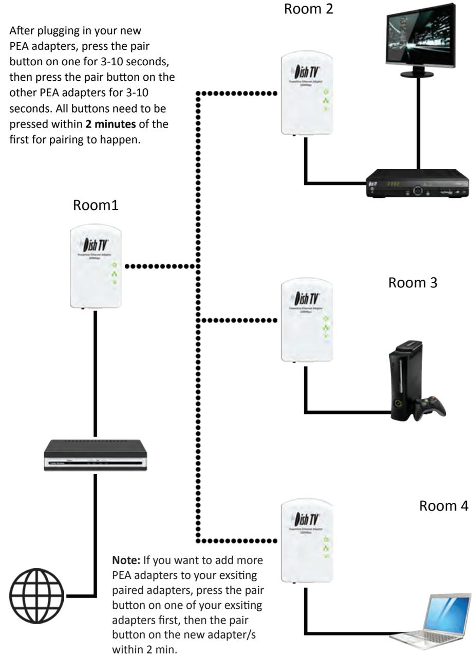
**Note:** If you want to add more PEA adapters to your existing paired adapters, press the pair button on one of your existing adapters first, then the pair button on the new adapter/s within 2 min.
