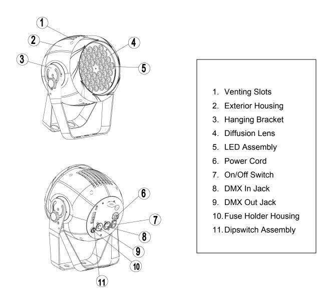
**1. Venting Slots –** These slots are designed to keep the fixture cool during operation. Never block these slots. Keep these slots clean at all times.
