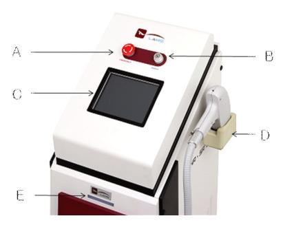
A. **Emergency Switch:** This is a switch for a user or an operator to stop the power source in unexpected emergency situations. If you push the switch, it will stop the power source and, if you want remove such stop to re-activate the product, you need to turn the switch to the right though the angle of 45 degree.
