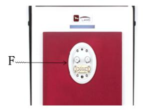
**F. Hand-piece Connector:** This is the place where the hand-piece and the product are connected with each other so that various sensors, power source lines and ultrapure cooling water are connected
