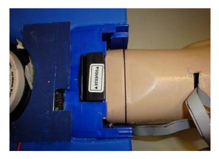
(3) Connect the cable of the head in the port of the torso.
