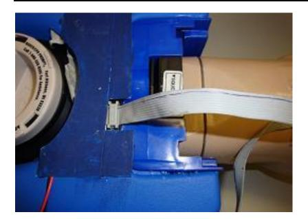
(4) Turn around the mannequin and connect the cable of the blue box in the blue port.
