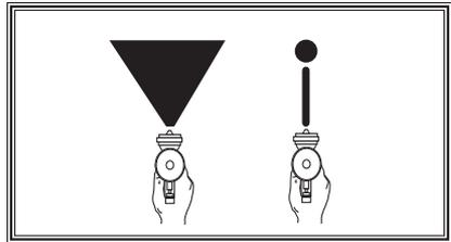
**Figure 9.** Fan adjustment.
