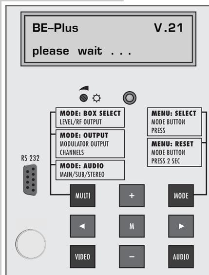
The transmodulator box is set up exclusively via the keyboard of the basic module carrier's control unit.
