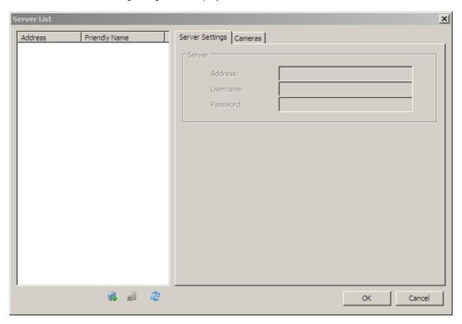
On the left-hand side of the window are two columns, *Address* and *Friendly Name*. The *Address* item contains the IP address or hostname that the Alarm Client uses to connect to the server. The *Friendly Name* item is an administrator-configurable name that is displayed to users whenever they must select a server from a list.
