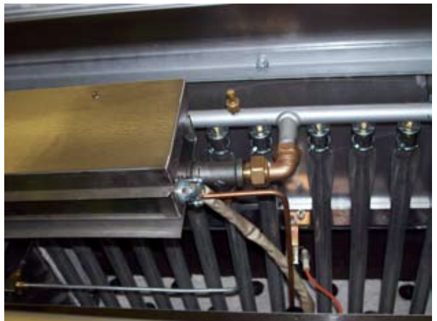
Fig. 7 Connect a gauge to check pressure at the gas manifold.
