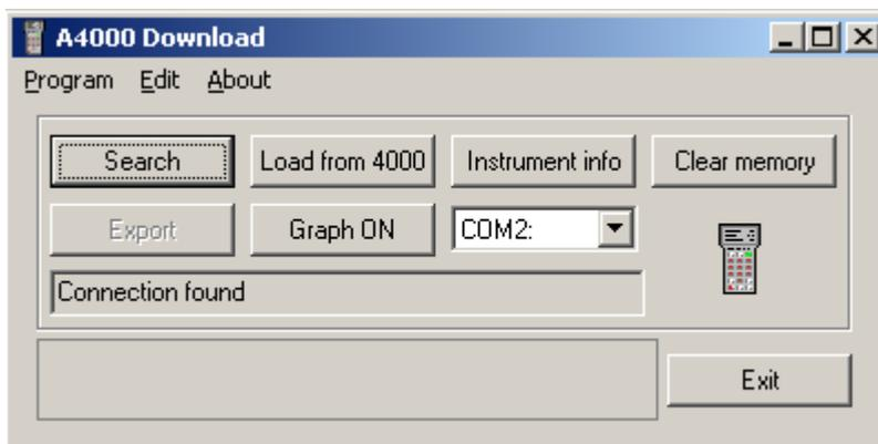
Fig. Connected instrument found by the program on COM2:
