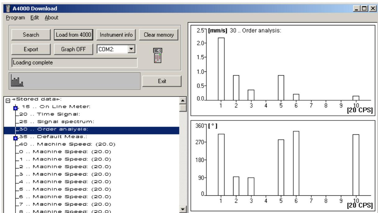
Fig. Graphic display of order analysis measurement results
