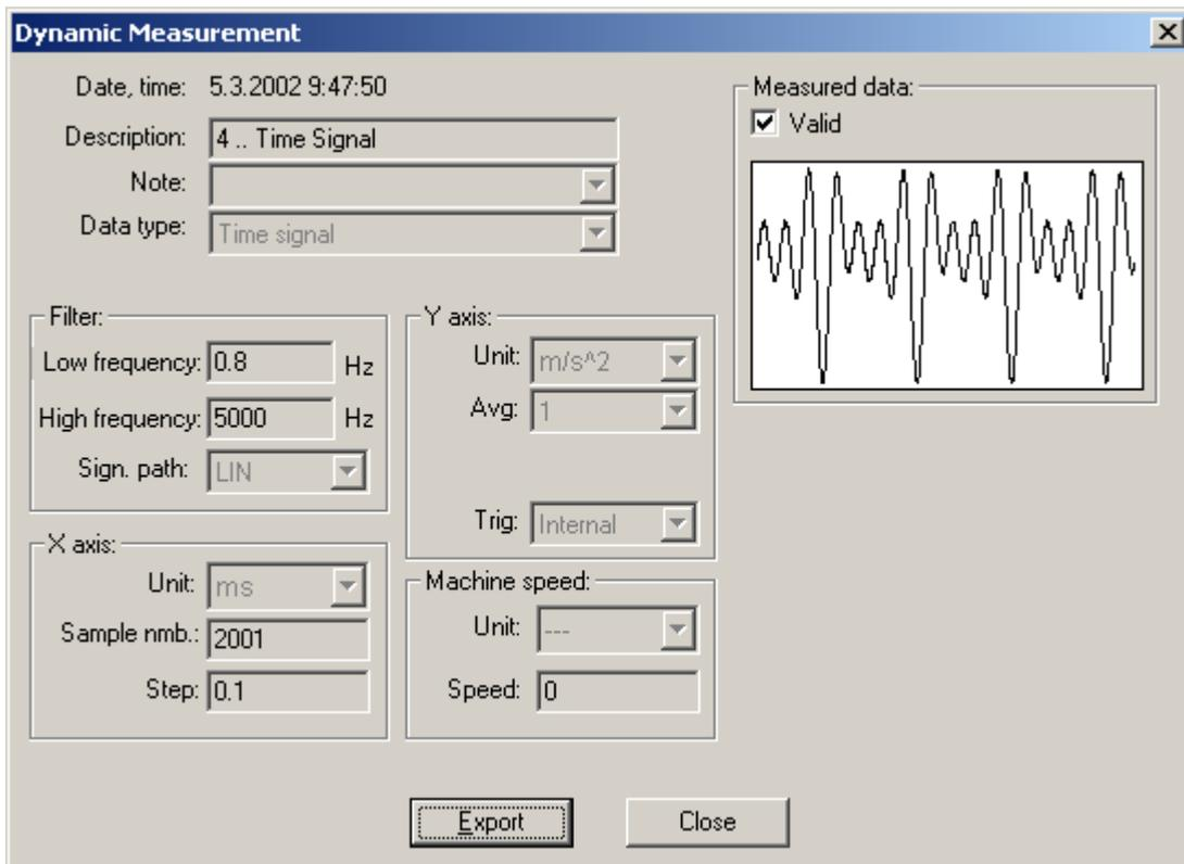
Fig. Information on time signal measurement
