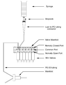
The VC-8M Valve Controller is assembled in the following manner:
