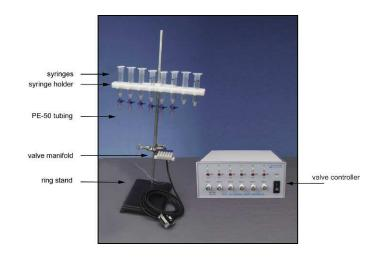
Next, attach the SYRINGE HOLDER to the RING STAND. Affix a LUER-TO-PE-50 TUBING connector to each STOPCOCK-WITH-LUER connector. Mount SYRINGES into the SYRINGE HOLDER and attach a prepared stopcock assembly to each SYRINGE. Now cut six (8) pieces of PE-50 tubing just long enough to run from the LUER-TO-PE-50 TUBING connector (on the SYRINGE) to the *input port* on each MINI-VALVE.
