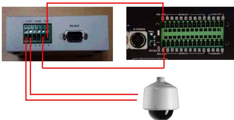
**Note** When you connect RS-485 cable, be careful for the polarity ((D+ → D+, D- → D-)).
