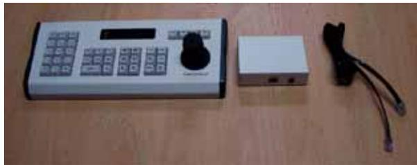
[Keyboard Controller, Junction Box and RS-485 Cable]
