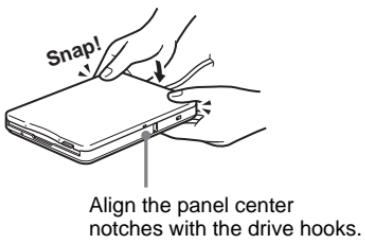
Align the panel center notches with the drive hooks.
