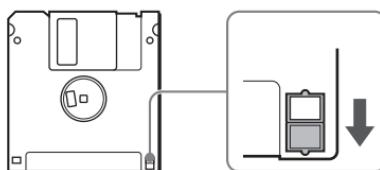
To remove the write-protection on a floppy disk, push the write-protect tab as illustrated below.
