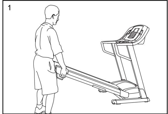
2. Move your right hand to the position shown and hold the treadmill firmly. Using your left hand, pull the latch knob to the left and hold it. Raise the treadmill until the frame is past the latch pin. Slowly release the latch knob. **Make sure that the frame is securely held by the latch pin.**
