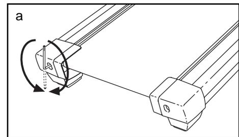
b. If the walking belt slips when walked on, first remove the key and **UNPLUG THE POWER CORD**. Using the allen wrench, turn both rear roller bolts clockwise 1/4 of a turn. When the walking belt is correctly tightened, you should be able to lift each side of the walking belt 3 to 4 inches off the walking platform. Be careful to keep the walking belt centered. Plug in the power cord, insert the key, and walk on the treadmill for a few minutes. Repeat until the walking belt is properly tightened.
