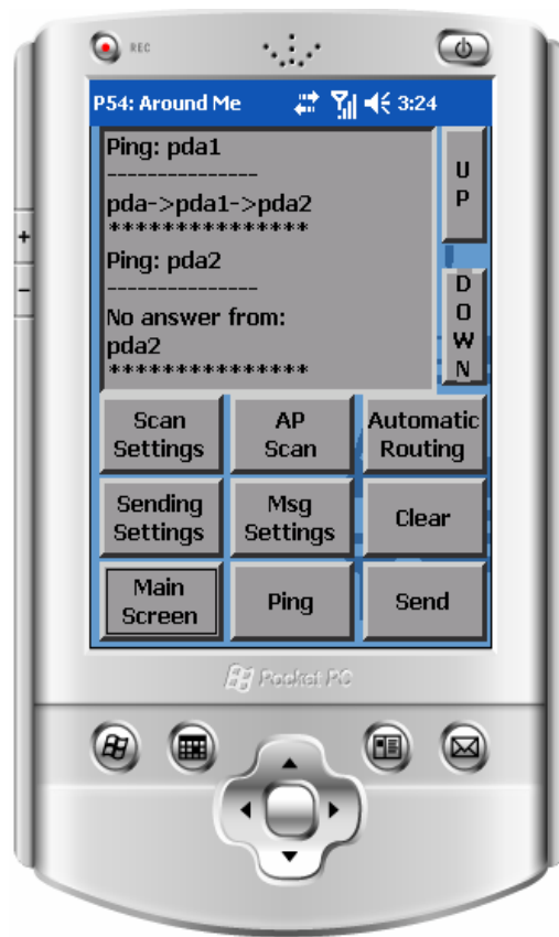
Fig 13: Example where there is no answer from PDA2, but PDA1 can see it.
