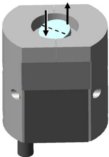
Figure 4: Maximum displacement in the positive direction of motion around axis 2. At the connected channel 2 of the amplifier, the output voltage U_{Piezo} is 100 V. The displacement shown is strongly exaggerated for better understanding.
