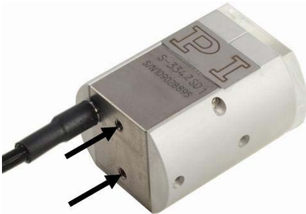
Figure 10: M3 holes of the S-334.2Sx1 for mounting on a surface and/or protective earth connection
