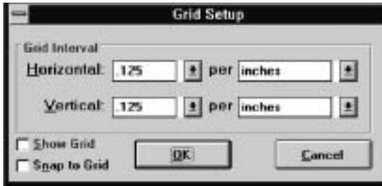
2. Enter or select the desired grid interval for the vertical and horizontal grid setup. The default grid setting is an eighth of an inch (.125").
