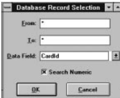
2. Select the **Data Field** from which you will be specifying the range of database records to be printed. *Example: If you wish to print a range of last names you have entered into Data Field 1, select Data Field 1 from the list of Data Fields.*
