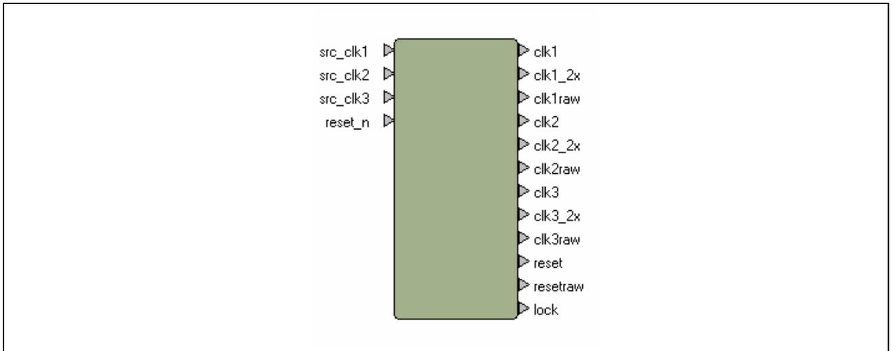
**Figure 39: Clock Driver Module Component - External**
