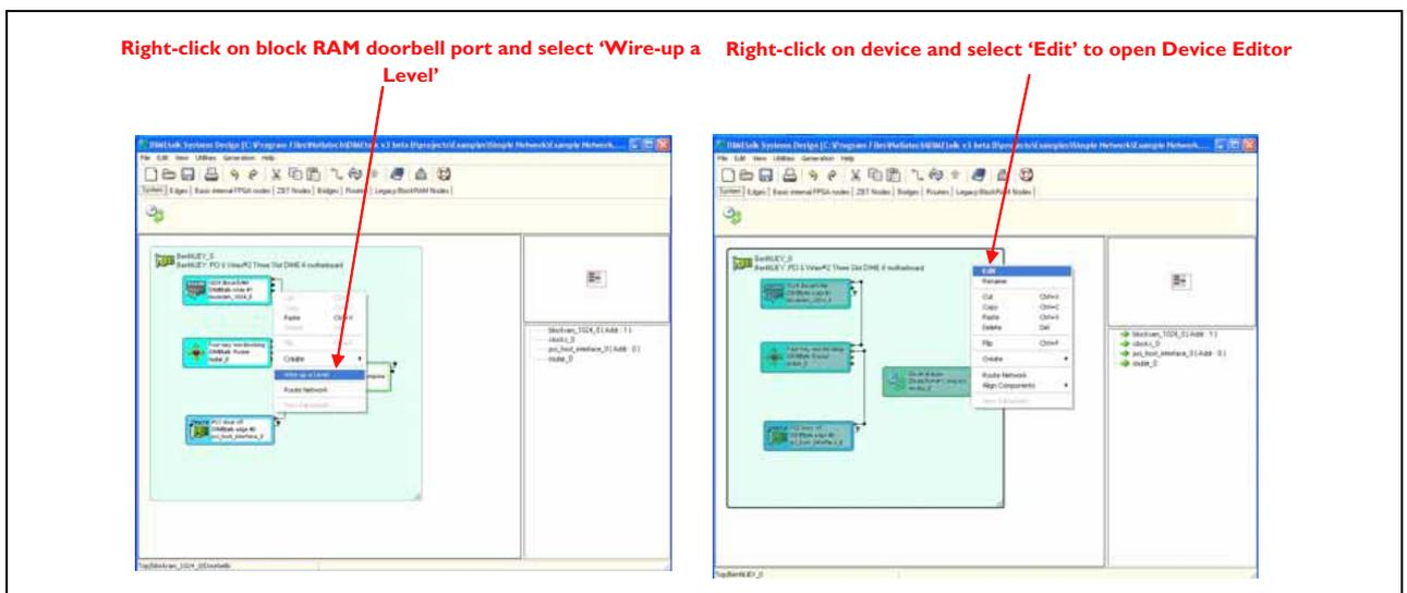
Figure 31: Assigning Signals to Pins
