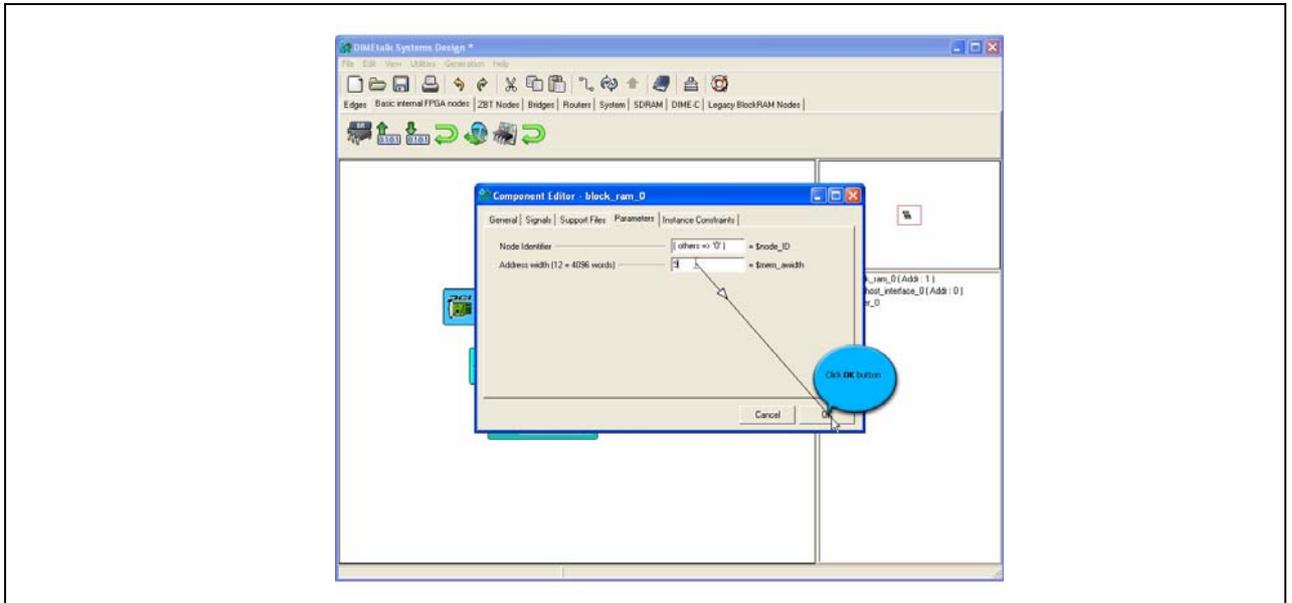
**Figure 9: Edit Block RAM Memory Address Width**
