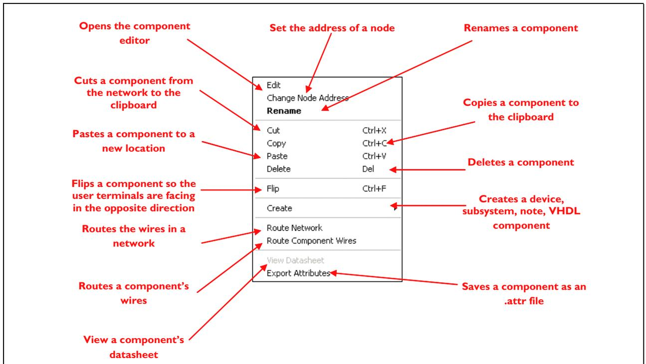
**Figure 28: Component Manipulation**
