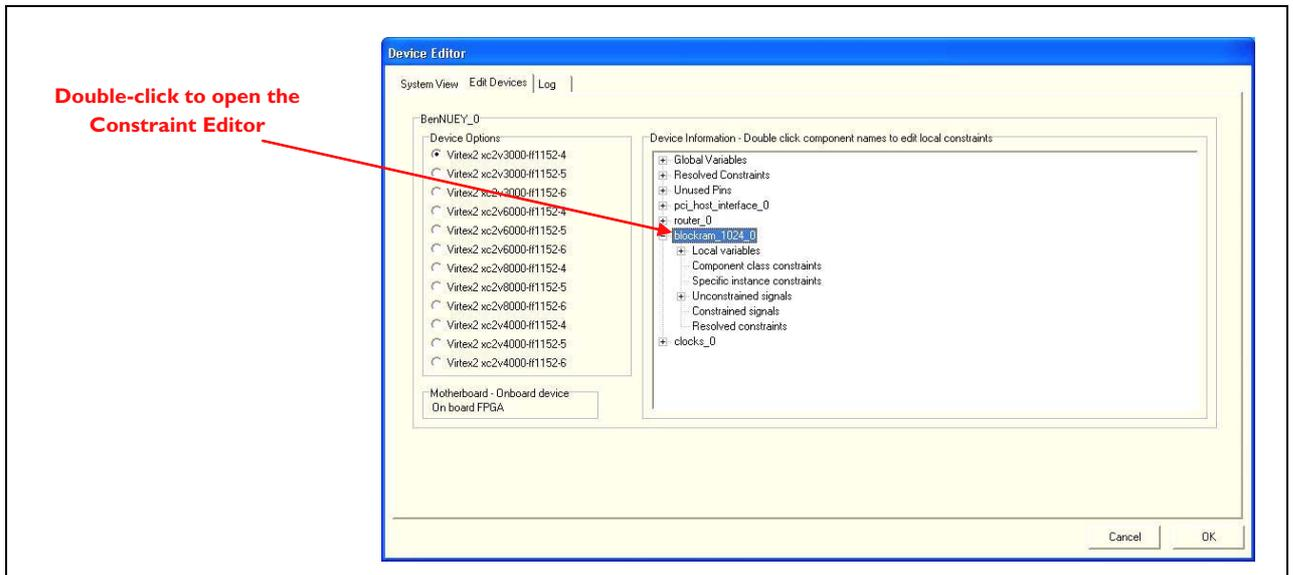
**Figure 32: Open the Constraint Editor**
