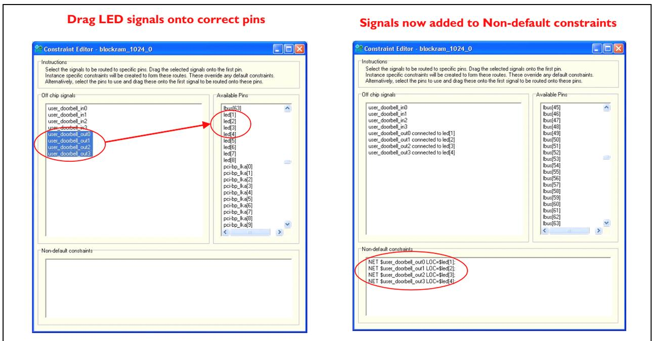
**Figure 33: Drag Signals onto Pins**
