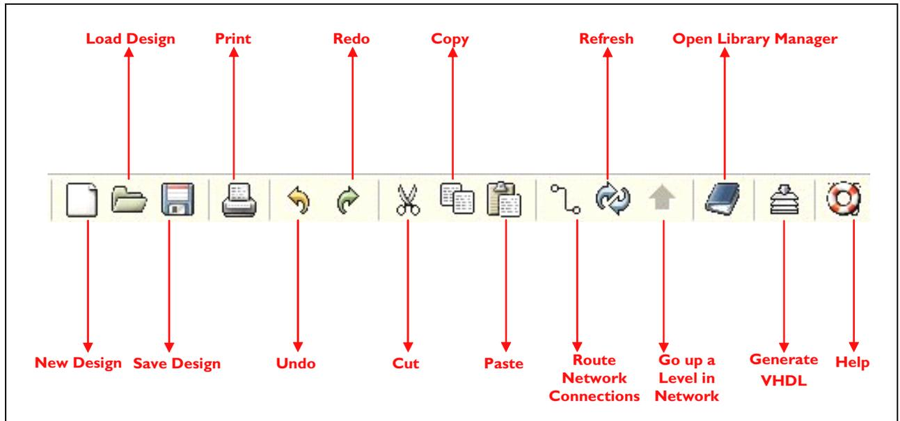
Figure 21: DIMEtalk System Design Toolbar
