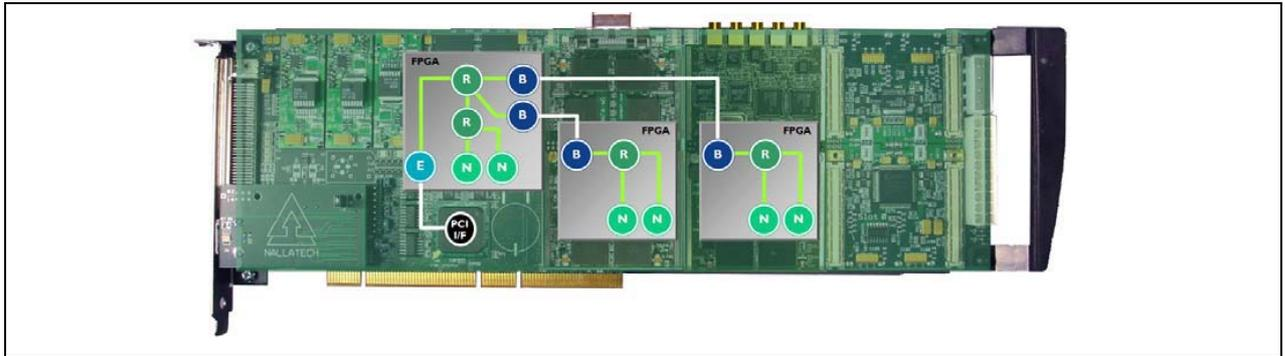
Figure 2: Example Multiple-FPGA Network
