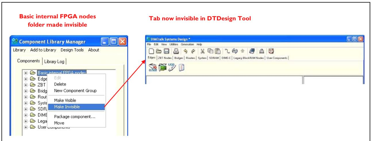
Figure 53: Make Component Tab Invisible
