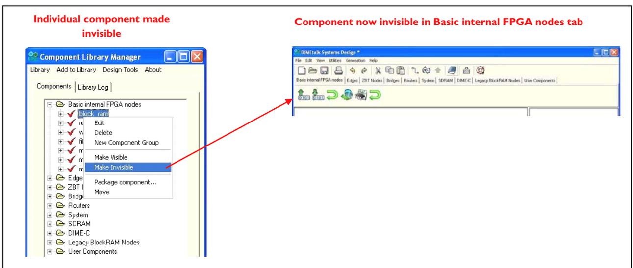
Figure 54: Make Individual Components Invisible
