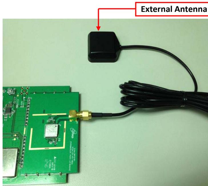
**b. Connect External Antenna with GPS Module.**
