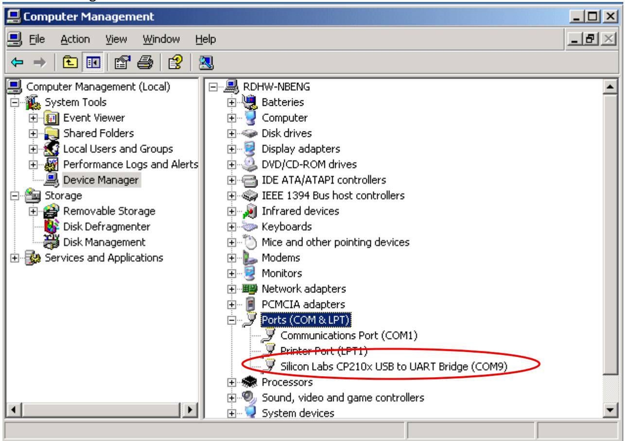
COM9 in this example represents the virtual COM Port number generated for the USB connection to EV-Kit.
