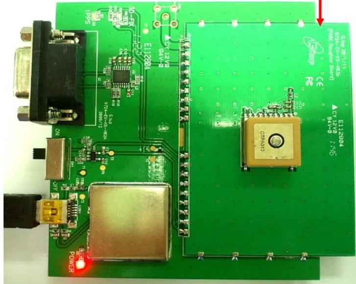
d. Using Chip Antenna with GPS Module as model below.
