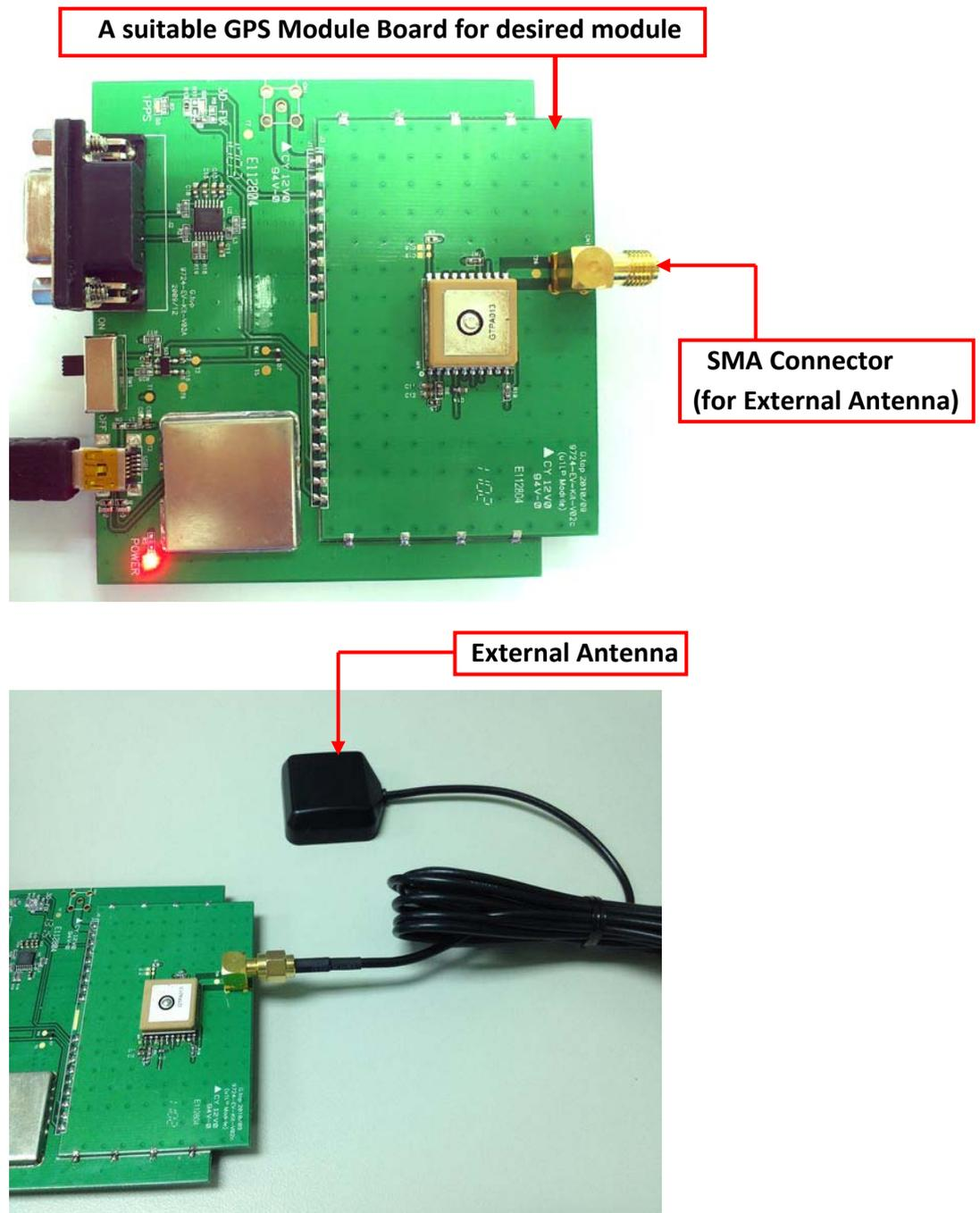
c. Connect Patch Antenna with GPS Module below.
