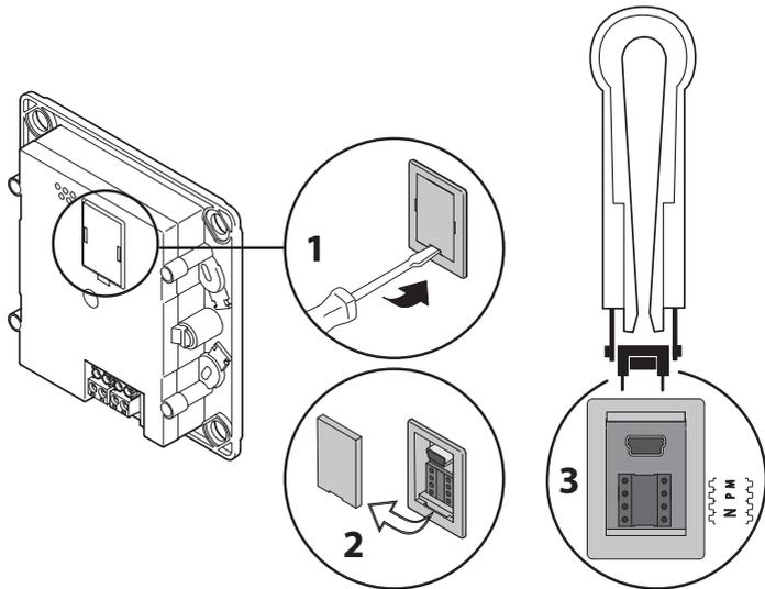
**N** = (in double figures) address of the device in the video door entry system
