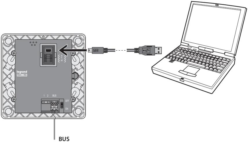
**In order for the communication to occur, the Video Display must be powered and not physically configured.**
