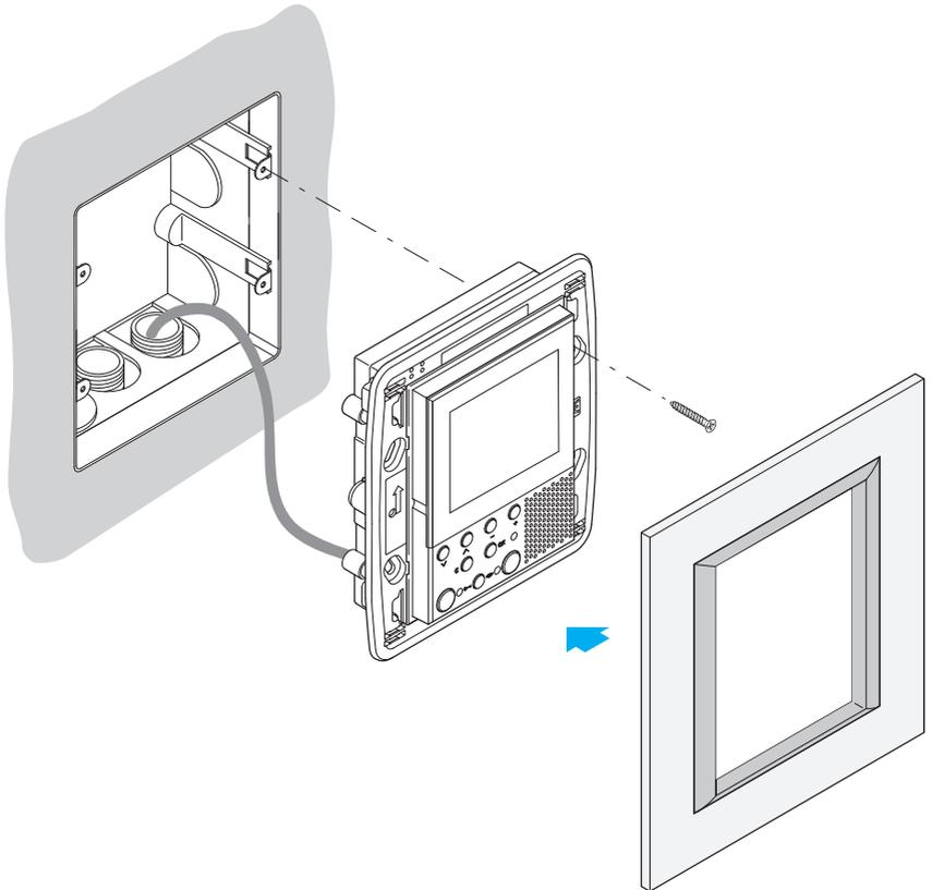
After making all the connections fasten the Video Display to the flush-mounted box being careful to arrange the wires so that they are not damaged.
