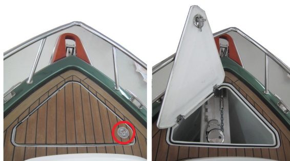
Picture 8: Anchor winch cover
