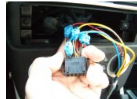
4. Completed connections, five splice clamps.
