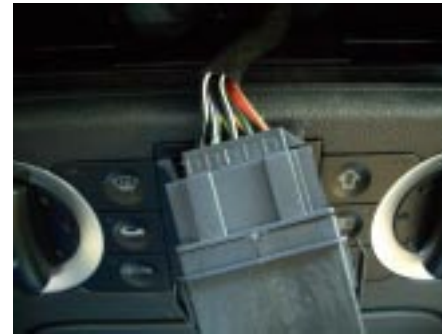
1. Disassembling the emergency switch, plug with pin numbers.
