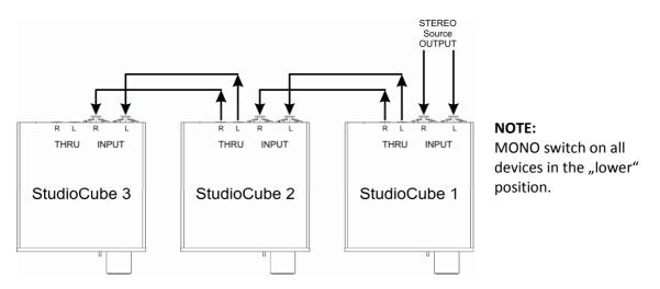
In some cases it can happen that there are not enough stereo channels available to act as source signals. The **StudioCube** can also be driven by a mono signal then. To avoid a single-sided channel reproduction in the headphone, the MONO switch must be activated.
