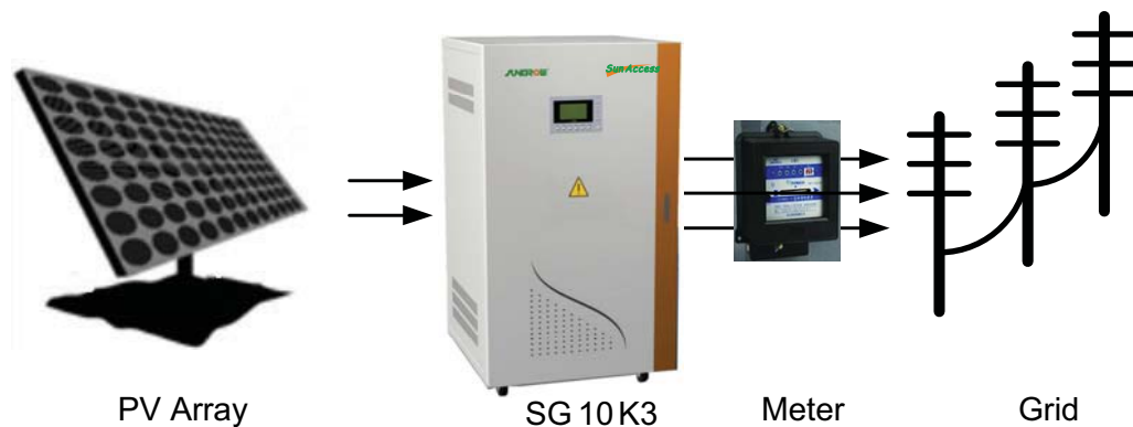
Fig.1 Grid-connected Inverter for PV power application
