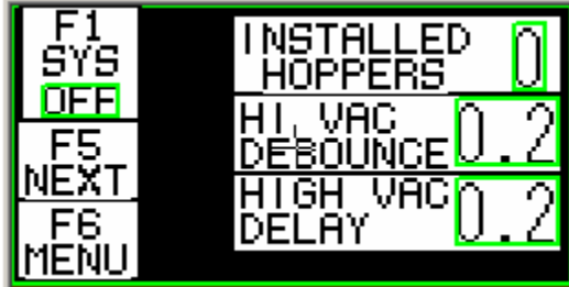
Figure 13: Initial System Setup Screen
