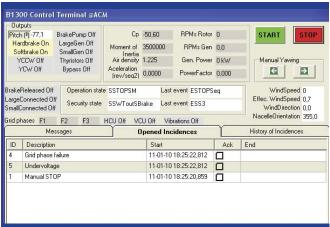
The various parts of this synoptic display as much information as possible to the user about the parameters values and a number of internal variables.
