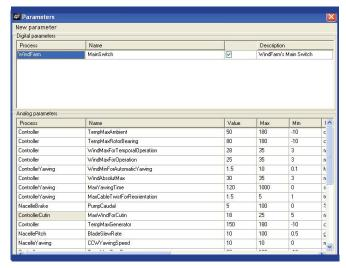
This synoptic is used to see and modify the Parameters values used in the application. Parameters behave as output signals or fixed value generators, either analog or digital.
