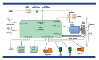
The connection of the generator to the grid while in production is direct. For the "cut-in" operation, the WT uses a set of thyristors for the connection of the generator to the grid during a short, controlled, period of time. The figure above shows the internal structure of a typical WT.
