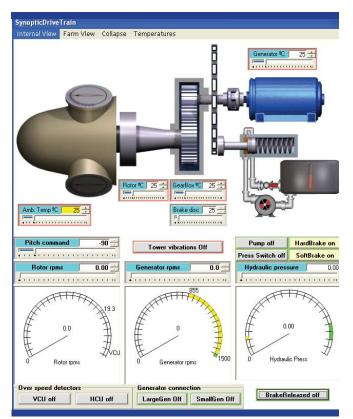
This WTDriveTrain synoptic has been designed to display the most important signals that arrive in the Nacelle emulator, and the signals going out from the Nacelle emulator.
