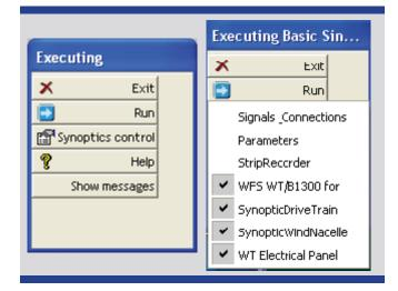
The Synoptics contain the HMI of the simulator associated with the configuration file. A synoptic element allows the user to visualize, in real time, the value of specified signals and to modify those values. Shown is the basic control synoptic of the WT Emulator. Default view is shown at left; expanded drop-down menu shown at right.
