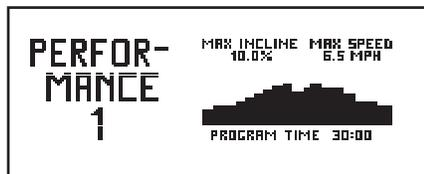
Each preset workout is divided into one-minute segments. One speed setting and one incline setting are programmed for each segment. Note: The same speed setting and/or incline setting may be programmed for consecutive segments.
