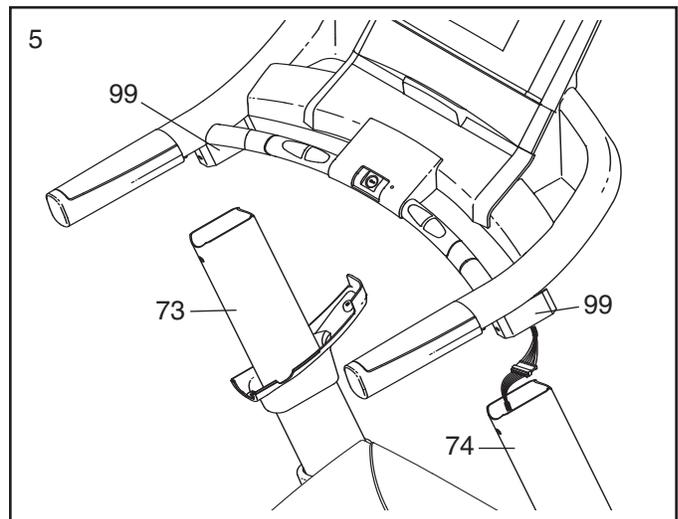
6. Finger tighten three Handrail Bolts (64) with three Star Washers (90) into the Right Upright (74). Next, finger tighten three Handrail Bolts with three Upright Star Washers (not shown) into the Left Upright (73). Then, firmly tighten the six Handrail Bolts.
