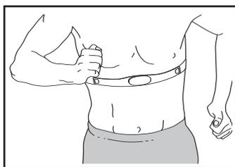
The chest pulse sensor should be under your clothes, tight against your skin, and as high under the pectoral muscles or breasts as is comfortable. Make sure that the logo on the sensor unit is facing forward and is right-side-up.
