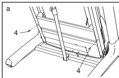
Lower the treadmill (see HOW TO LOWER THE TREADMILL FOR USE on page 24). Remove the four indicated 3/4" Screws (4), and remove the Hood (44).
