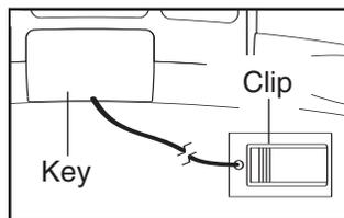
Then, insert the key into the console. After a moment, the displays will light. **IMPORTANT:** In an emergency situation, the key can be pulled from the console, causing the walking belt to slow to a stop. Test the clip by carefully taking a few steps backward; if the key is not pulled from the console, adjust the position of the clip.
