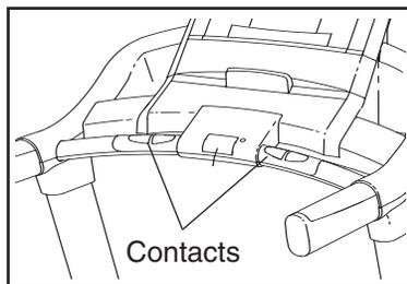
To measure your heart rate, **stand on the foot rails. Hold the contacts for approximately ten seconds—avoid moving your hands.** When your pulse is detected, your heart rate will be shown. **For the most accurate heart rate reading, continue to hold the contacts for about 15 seconds.**
