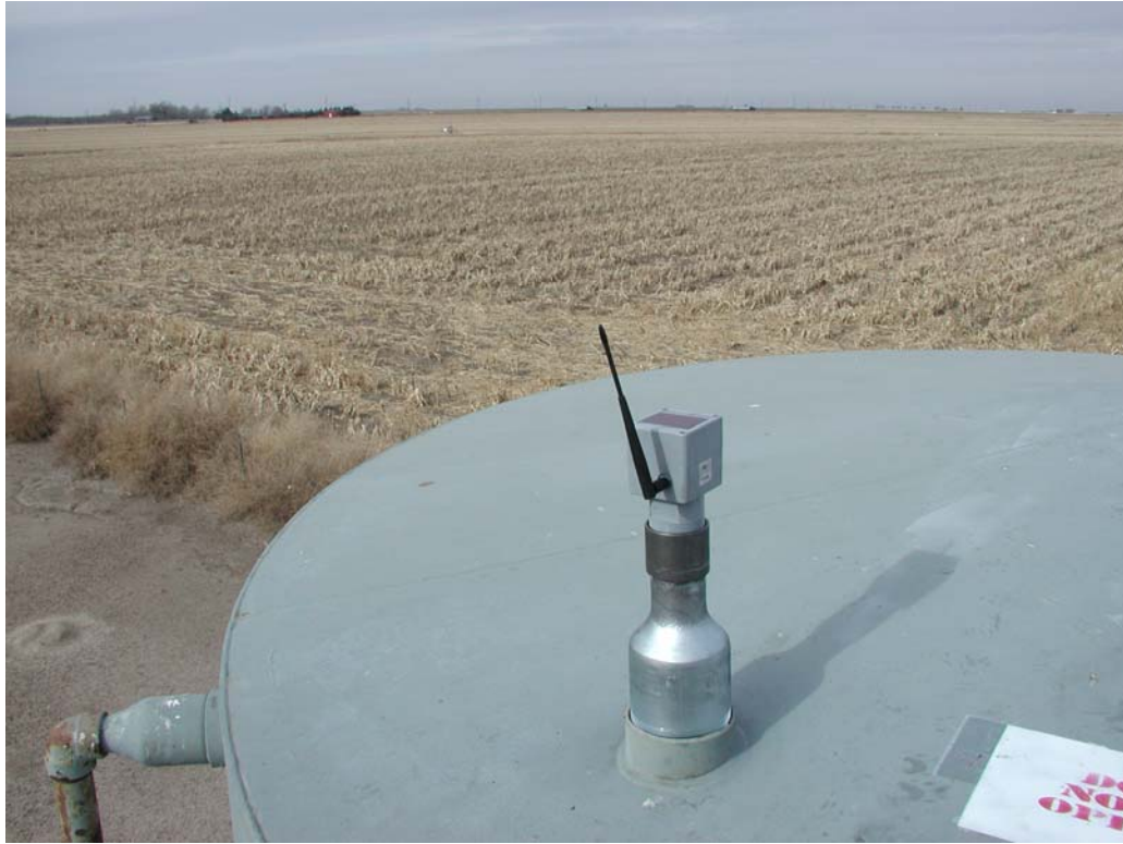
Figure 3. Preferred mounting method on a 2" NPT non-vent pipe.
