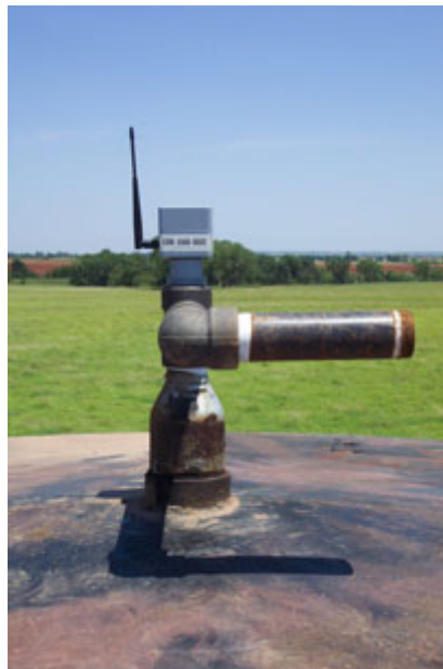
Figure 4 Mounting on a 2" NPT vent pipe.
