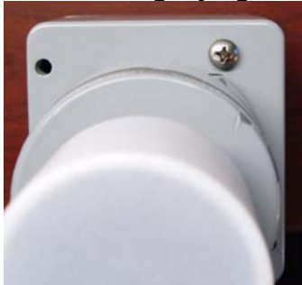
Figure 5. Reset button access screw.
