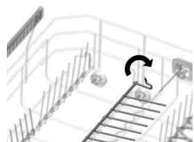
Anti-drip inserts which improve the drying of dishes. They may be supplied fitted on the basket or in the accessories bag; in this case, to use them, simply fit them into place as shown.
