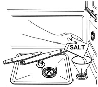
When using water of medium hardness, the regenerating salt container should be refilled after approximately **20 washing cycles**. The salt container can hold approximately **1.7 Kg** of salt in grains. The container is situated at the bottom of the dishwasher. After removing the lower basket, unscrew the salt container cap by turning it anticlockwise and pour in the salt using the funnel supplied with the dishwasher. Before replacing the cap, remove any salt residues from around the opening.
