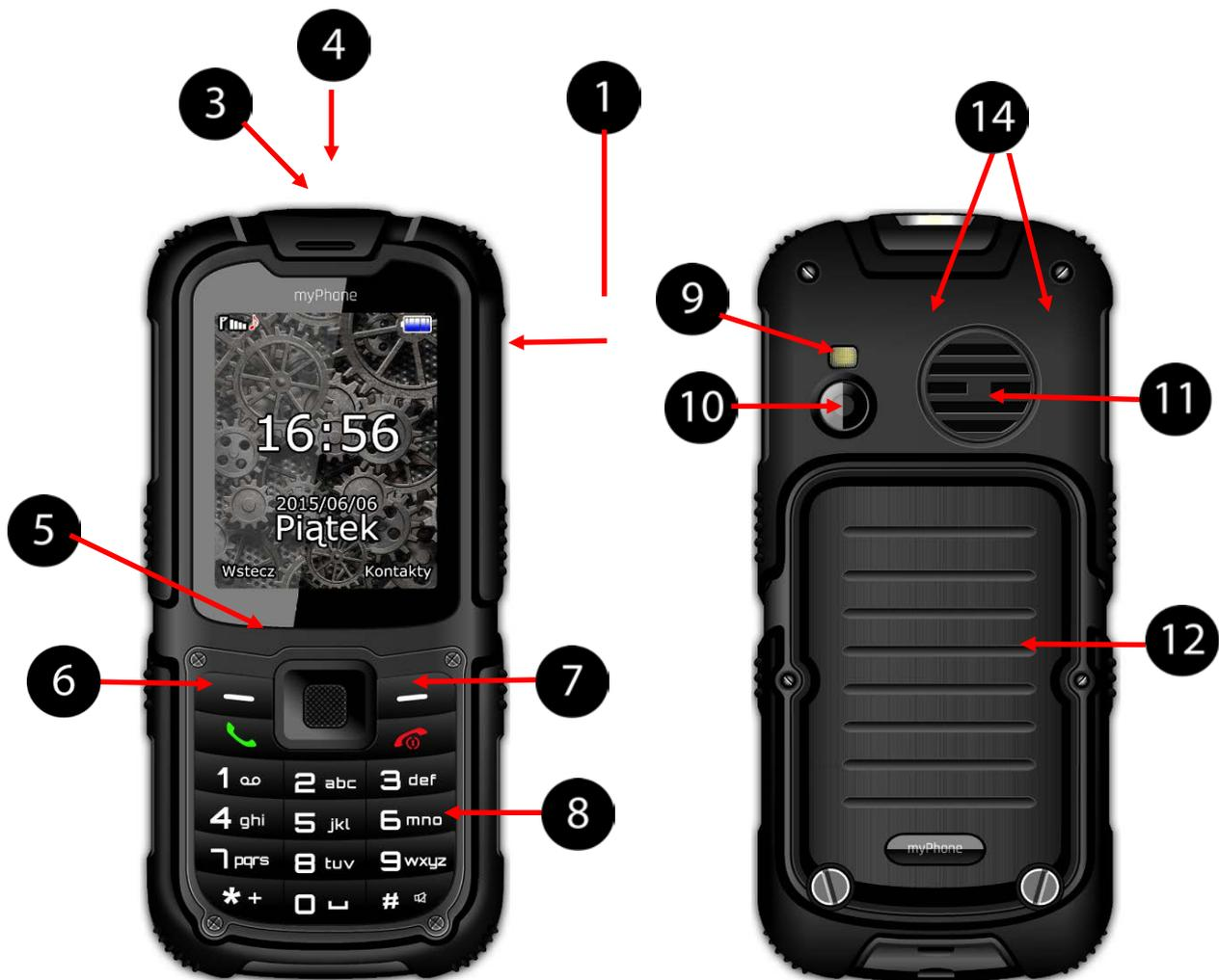
1. microUSB port (under the rubber plug).
