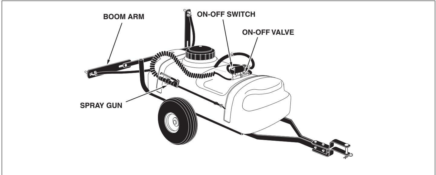
**ON-OFF SWITCH** Turns pump/motor on or off.
