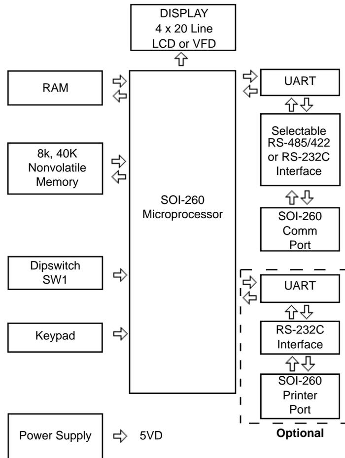
Figure 2.2 SOI-260 Functional Block Diagram
