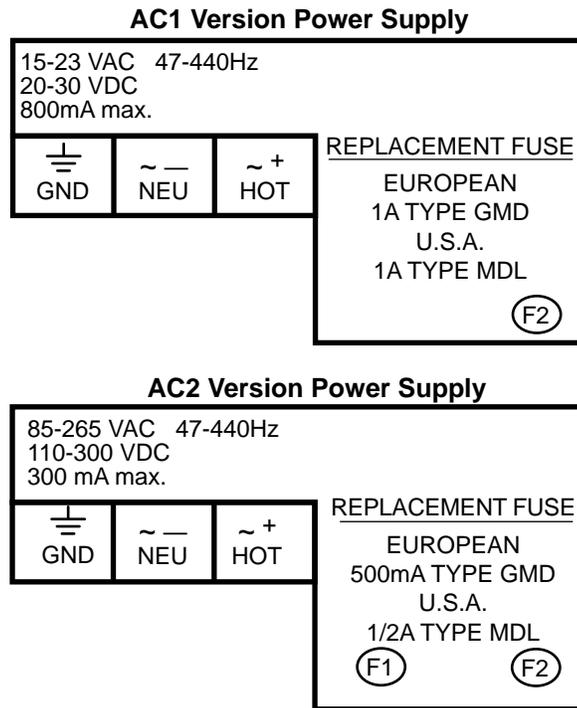
Figure 2.4 AC1 and AC2 Power Supply Connections
