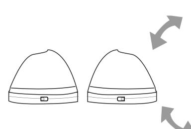
Hold onto the top of the speaker and twist anti-clockwise to reveal the resonator.
