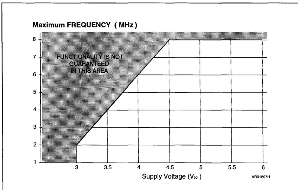
Note: The shaded area is outside the recommended operating range; device functionality is not guaranteed under these conditions.
