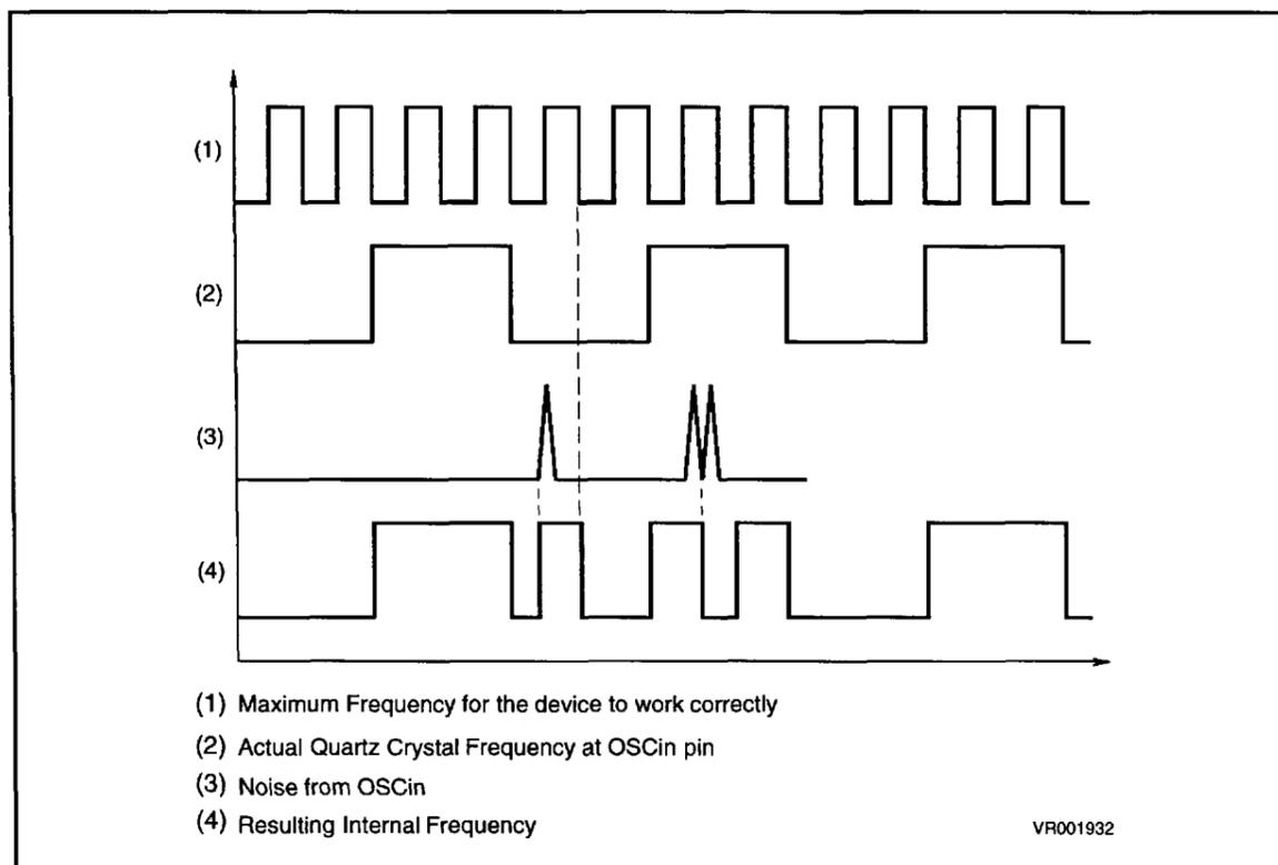
Figure 13. OSG Emergency Oscillator Principle
