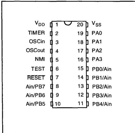
Figure 4. ST6215B, ST6225B Pin Configuration
