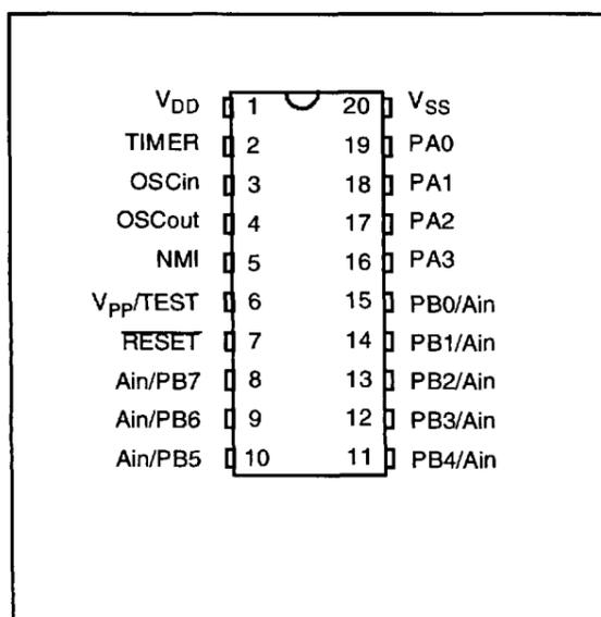
Figure 3. ST62T15, T25, E25 Pin Configuration
