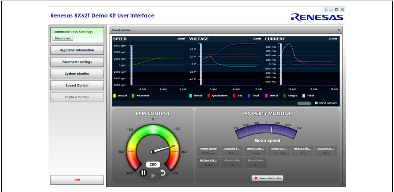
Figure 28 Setting the Speed to Turn the Motor in the GUI Application
