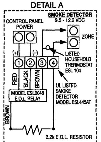
\* UL INSTALLATIONS REQUIRE LISTED END-OF-LINE DEVICE. USE RESISTOR FROM EOL22 KIT. LOOK FOR LISTING MARK ON ITEM.
