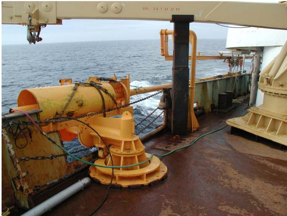
Figure 3. GSCA large diameter piston corehead with 30 ft. of core barrel and FFCPT. Tests were conducted with as much as 50 ft of core barrel.
