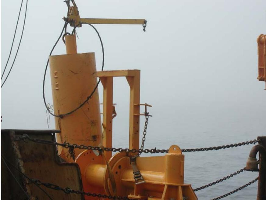
Figure 5. Trip arm attached to the wire and the piston corehead, with 8 ft of free fall (note loop in recovery wire). The end of the recovery wire is attached to a sliding piston inside the core barrel, which allows the system to fully penetrate the seabed.
