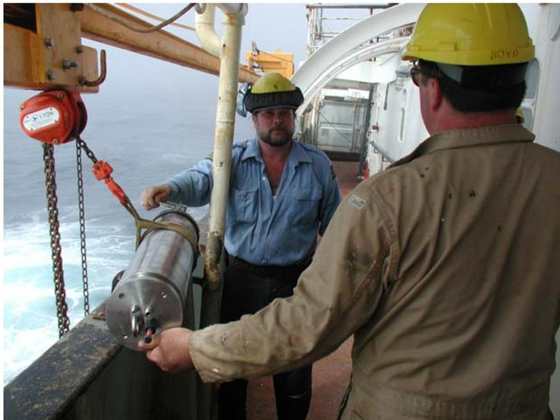
Figure 1b. Mounting the FFCPT on the end of the GSCA large diameter piston corer at the rail, in preparation for deployment.
