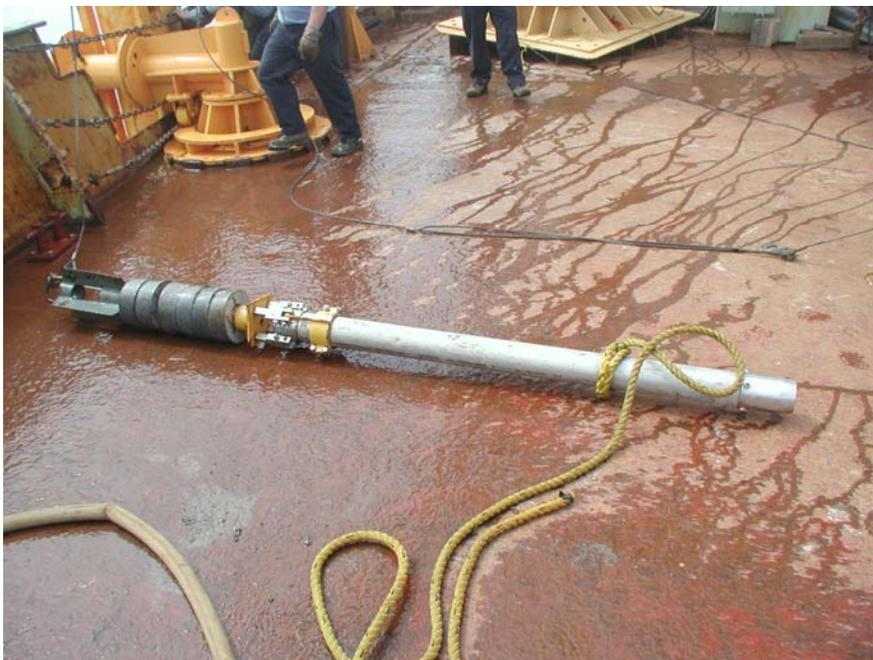
Figure 6. 3m gravity corer being attached to the end of the trip arm wire. This allows for release of the piston corer into free fall at the correct height (free fall distance) above the seafloor. A small sample is collected each time this corer is used.
