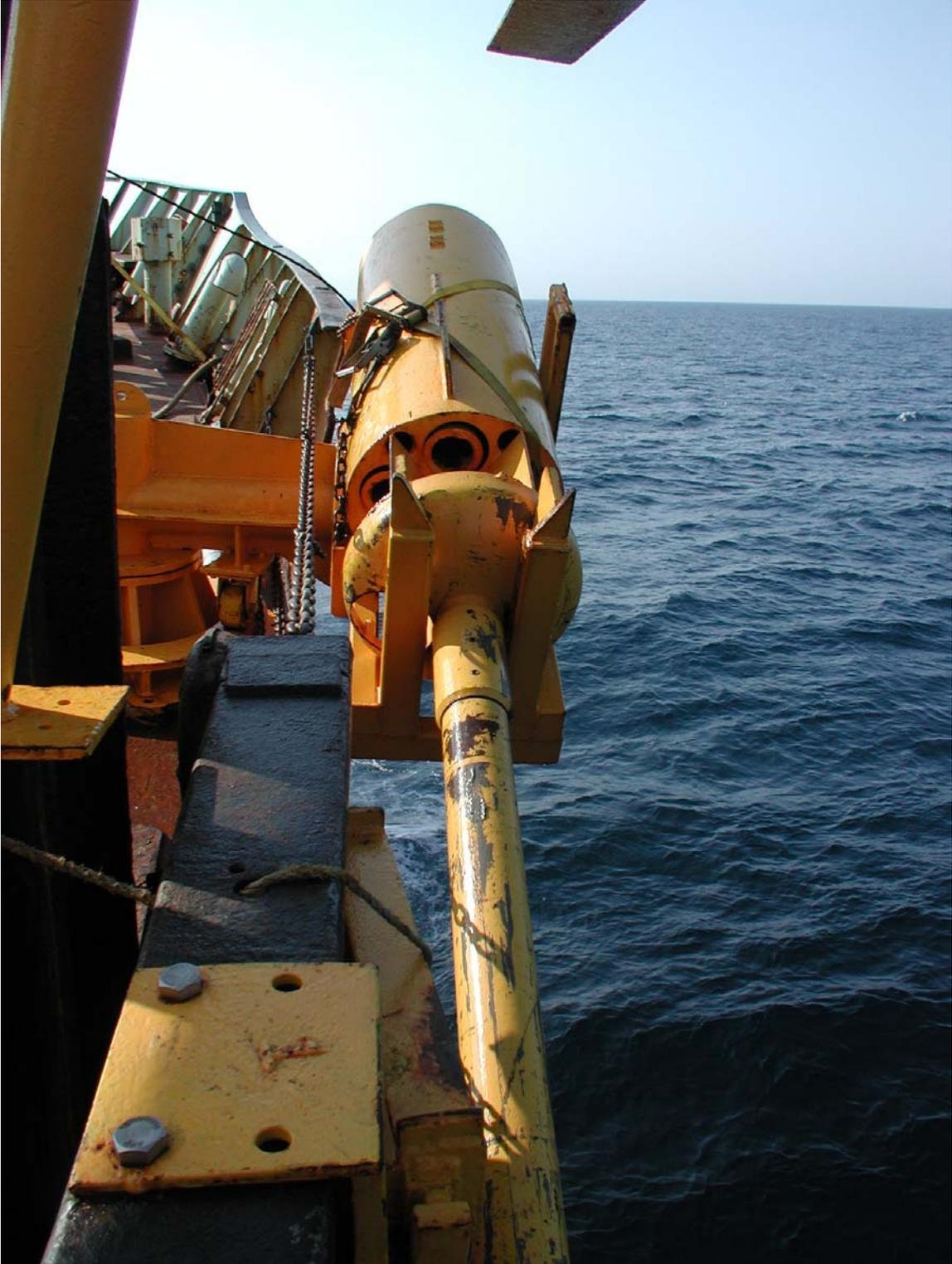
Figure 4. GSCA large diameter piston being rotated to a vertical position.
