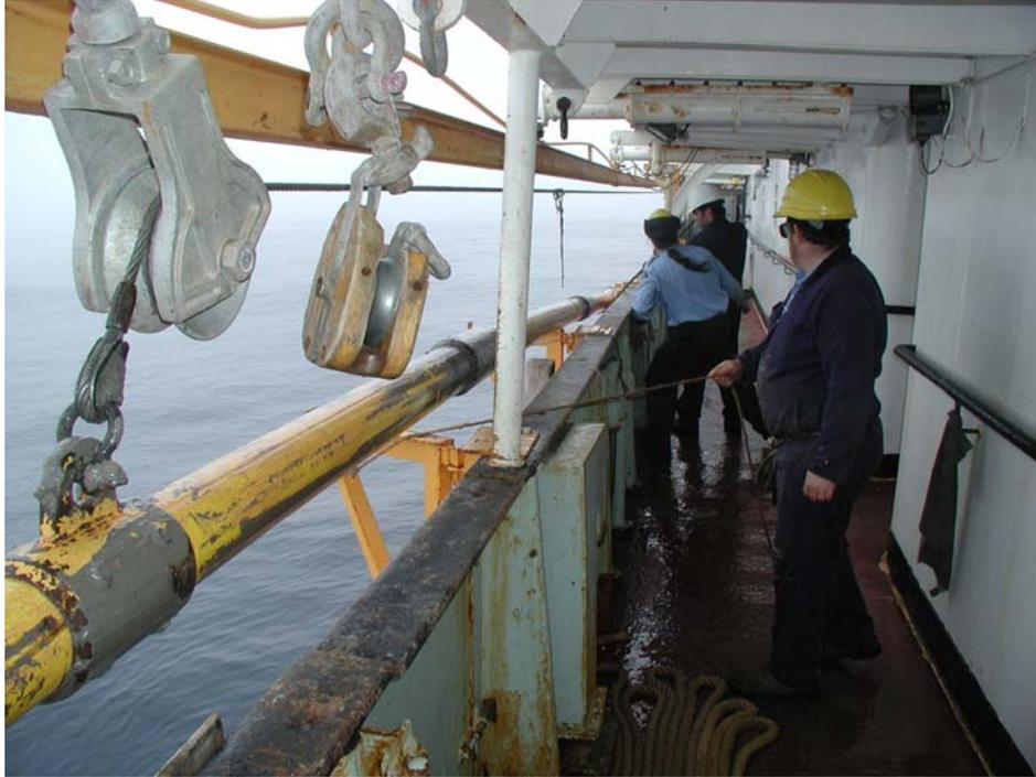
Figure 7. FFCPT and 50 ft. of core barrel being raised to the rail. CCG Hudson can accommodate as much as 100 ft. of core barrel, using the dedicated monorail system (see top of photo).
