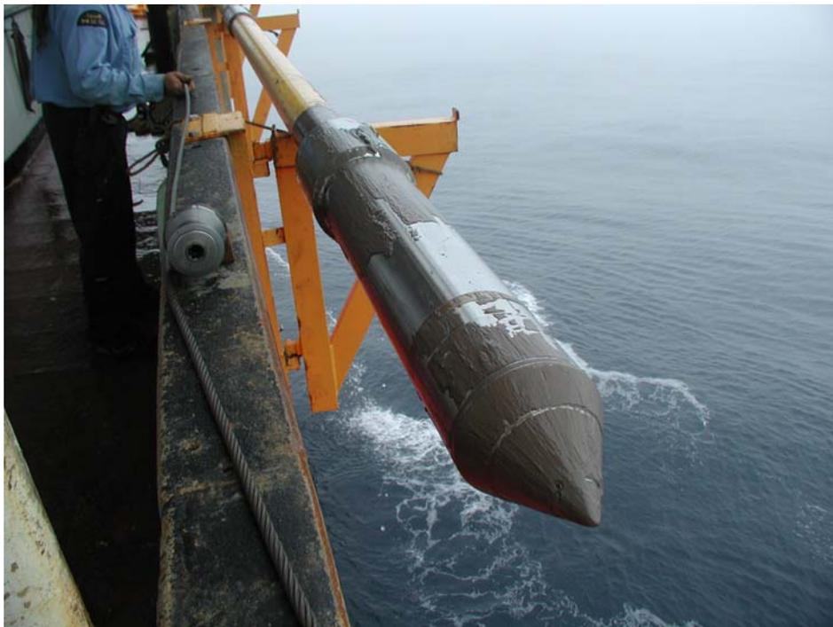
Figure 8. FFCPT after recovery, showing mud up to the split coupling on the core barrel, before being pressure-washed.
