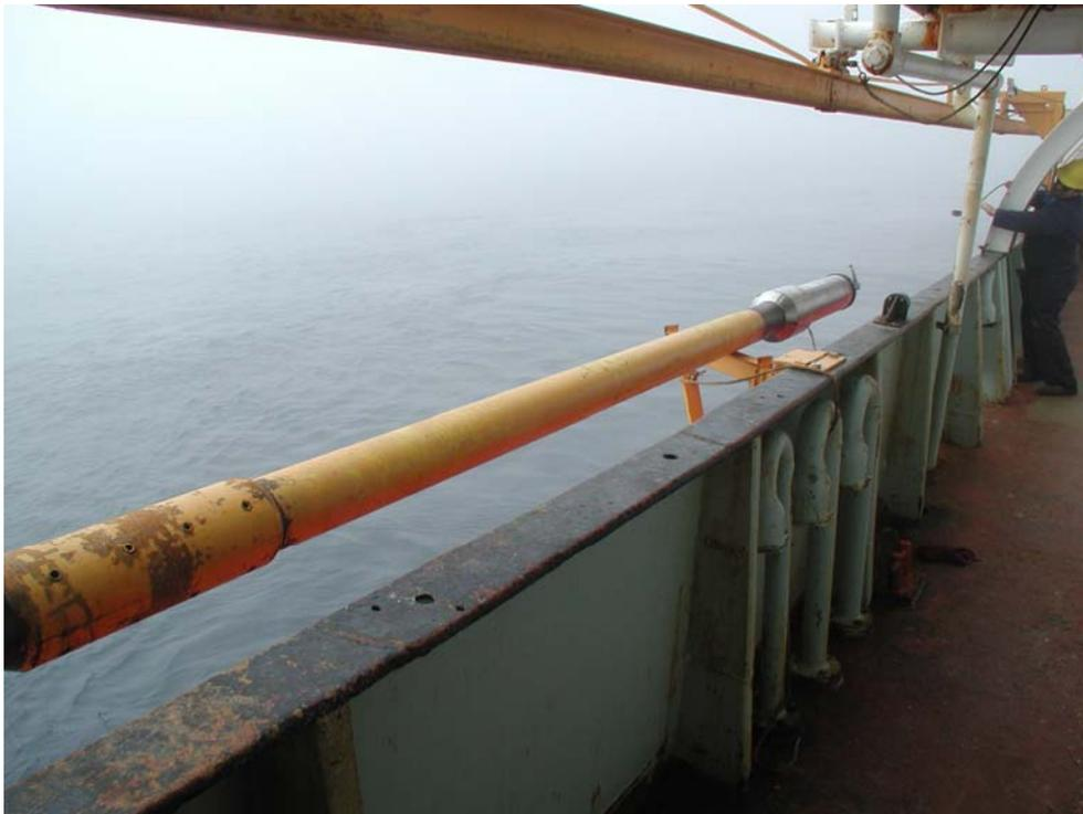
Figure 2b. FFCPT on core barrel, ready for lowering.
