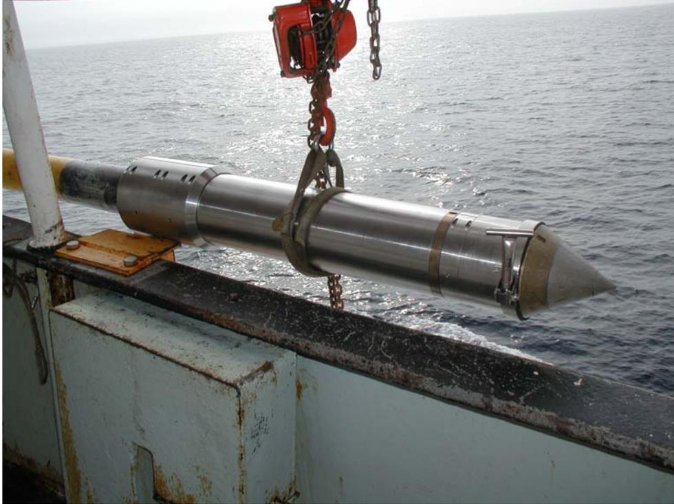
Figure 2a. FFCPT Mounted on the end of the GSCA large diameter piston corer at the rail, in preparation for lowering.
