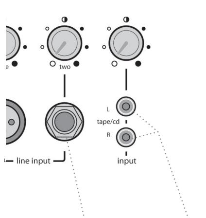
Plug any line-level source with a 1/4" phone plug (tape player, music instrument, etc) into line input two. The knob above the jack controls the volume level.
