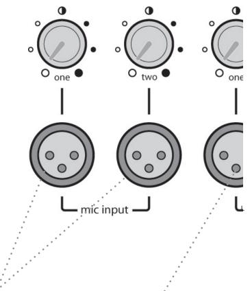
Plug a microphone with an XLR connector into mic input one or two. The knob above the jack controls the volume level.
