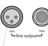
Connect line output one to the balanced input of another system for daisy-chain applications.
