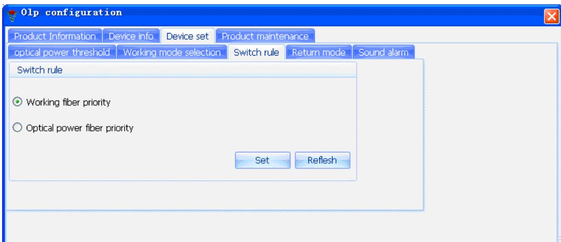
d) Return Mode includes two types: manual return and automatically return (it is workable for 1+1 type OLP device). Shown as below:
